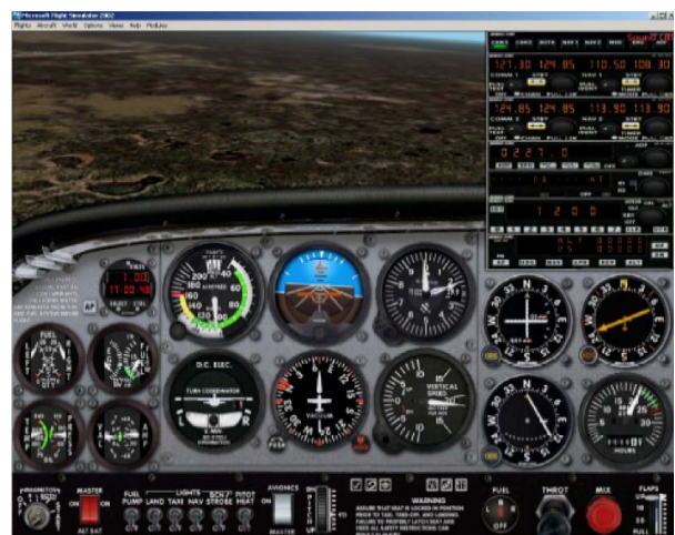
Figure 9. A traditional cockpit display
